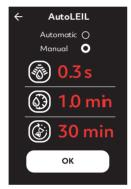
The exact amount of water dispensed depends on the water tap pressure. Please note that in most cases with good water pressure 2–4 second value for water quantity can be an excessive amount of water. We recommend start testing with 0.5–0.8 sec to get a feel.
